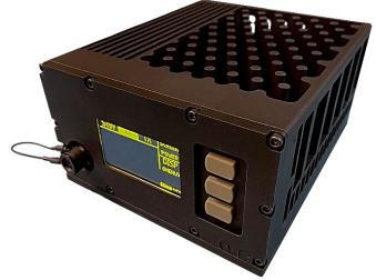
The following specifications apply to the **AR Modular RF** booster model **AR-FS-20U** – a standard amplifier providing **20 Watts** output power from **225 to 450 MHz** with pass-through support outside of this band.
