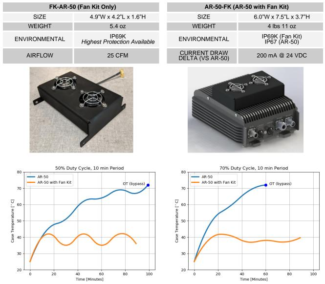
Testing performed at 25°C ambient, laboratory environment. As the plots illustrate, fan kit forced convection cooling significantly increases the efficiency of the AR-50, allowing it to operate indefinitely, without reaching over temperature (OT) conditions.
