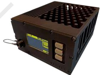
The following specifications apply to the **AR Modular RF** booster model **AR-FS-20LS** – a standard amplifier providing **20 Watts** output power from **1250 to 2600 MHz** with pass-through support outside of this band.
